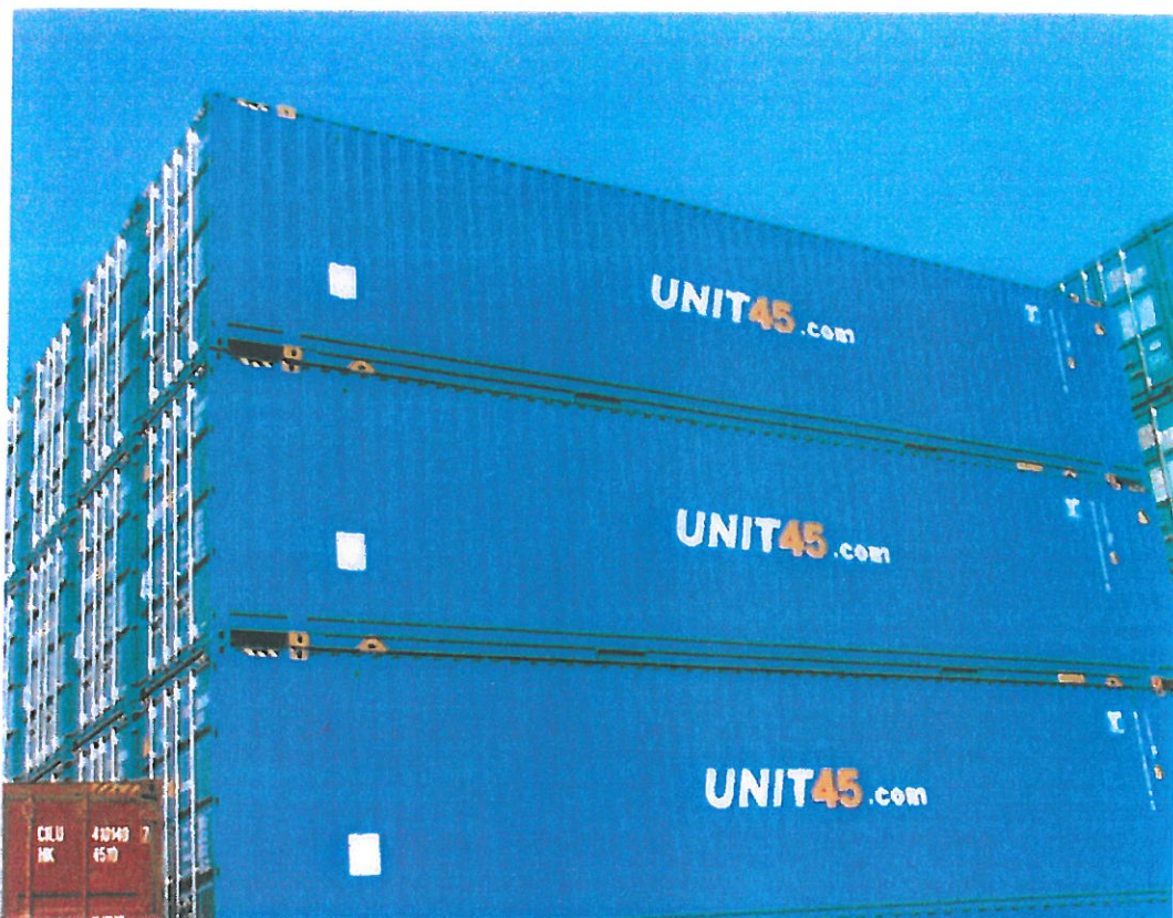
Unit 45 containers are capable of carrying 33 Euro pallets, giving them a capacity of up to 25% more than ISO 40ft boxes
